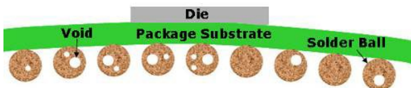
Figure 16 — Diagram of a Warped BGA Package
